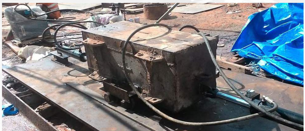
Pengetesan Steering Gear Project Kapal Rede Kemenhub. PT Daya Yes Shipyard
